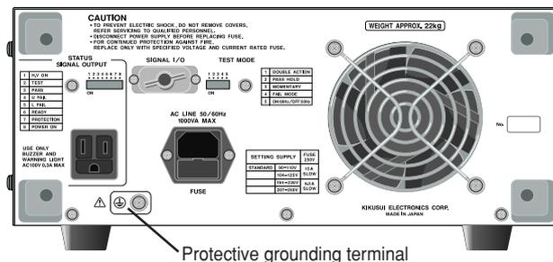
Figure 1-3 Protective Grounding Terminal
