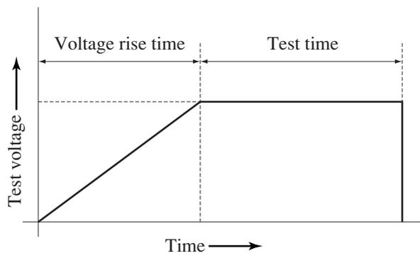
Figure 3-1 Voltage Rise Time and Test Time
