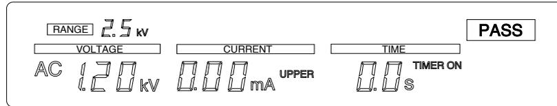
This display indicates that the measured voltage is 1.20 kV, that the measured current is 0.00 mA, and that PASS is appeared.
