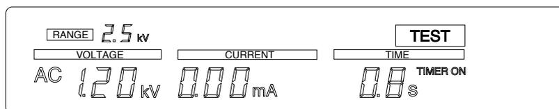
This display indicates that the measured voltage is 1.20 kV, that the measured current is 0.00 mA, and that the remaining test time is 0.8 s (The elapsed time is indicated in the TIME display when the timer function is held off).
