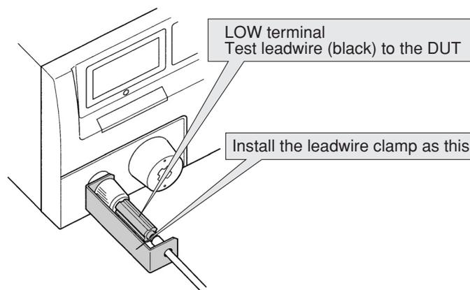
Figure 3-2 Connecting the low-voltage side test leadwire
